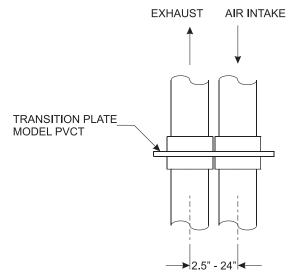
In both vertical and horizontal colinear direct vent applications, a colinear transition plate model PVCT can be used to minimize clearances between intake and exhaust pipes.
